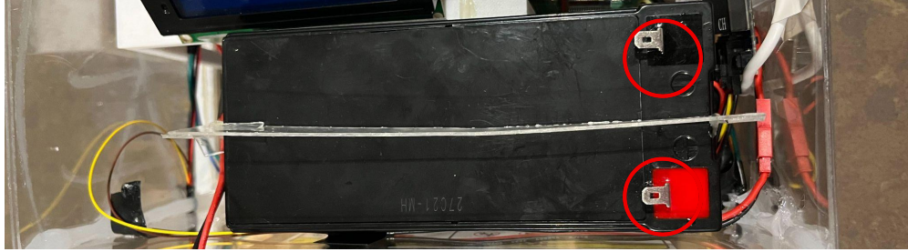
(Figure 2: 12V Battery's Terminal Connection)
