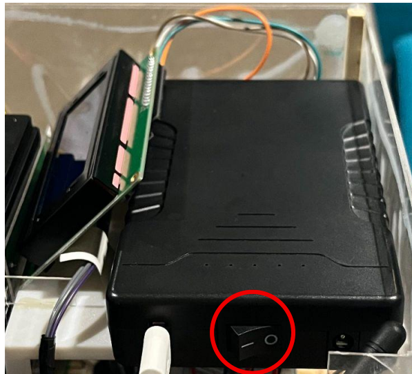
(Figure 1: Battery Pack Switch for RaspberryPi)
